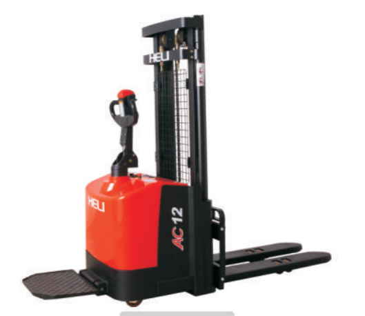
CDD12-030 1200Kg Narrow Legs /2-Stage Mast
