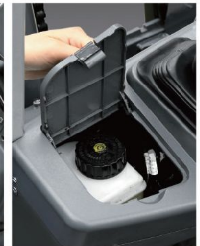
Brake fluid within reach, easy to check and refill
