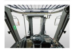
Excellent front view which is benefit for the work safety improvementand working efficiency is provide with wide view mast which hasproprietary intellectual property and fork positioner with side shifting.
