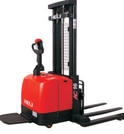
CDD16-D920 1600Kg Wide Legs/2-Stage Mast
