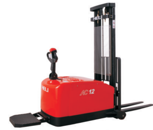
CDD12-970 1200Kg Counterbalanced /2-Stage Mast
