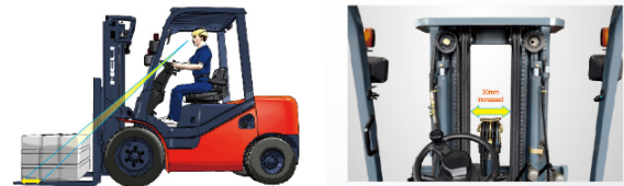
• visibility at the fork tip and goods 20mm increased • front view 30mm enlarged
